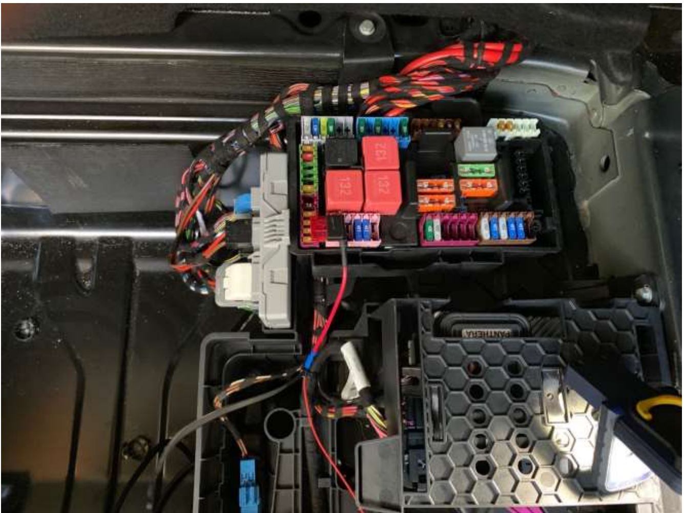
Example Image: Fuse Box Mercedes W205 C-Class
